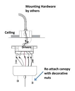
Before starting the installation, unscrew the two decorative nuts of the Driver Housing (factory provided). Then loosen the two nuts (Factory provided) holding the Driver Assembly with the Canopy.
