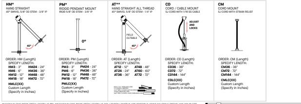
\*MAXIMUM ONE PIECE STEM LENGTH IS 72". \*\*MAXIMUM ONE PIECE STEM LENGTH IS 36", LONGER LENGTHS ARE POSSIBLE USING MULTIPLE STEMS AND COUPLERS. \*\*ORDER IN 12" INCREMENTS, ODD SIZES MAY BE FIELD CUT
