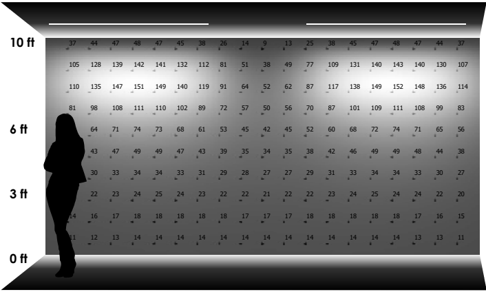
TWO LUMINAIRES 2'-0" away from wall 10'-0" on center
