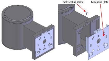
Remove Mounting Plate by taking out self-sealing screw.
