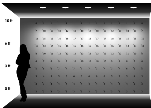
5 LUMINAIRES 3' away from wall 3' between luminaires
