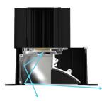
The system provides high (close to ceiling) even illumination for vertical surfaces with superior room side glare control. The measured performance of the system is extremely efficient, with the most even distribution vertically and horizontally in its category.
