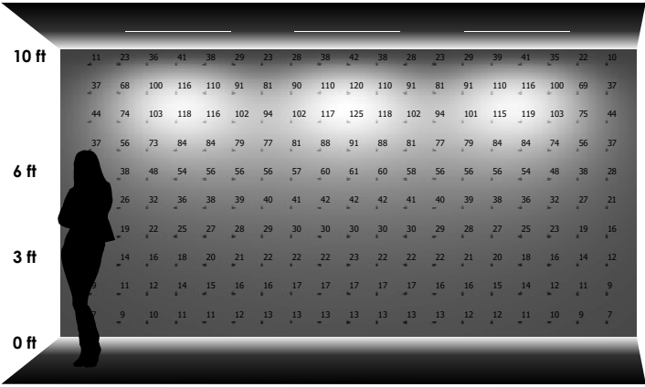
THREE LUMINAIRES 2'-0" away from wall 6'-0" on center
