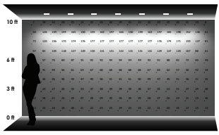
SEVEN LUMINAIRES 2'-6" away from wall 2'-6" between luminaires
