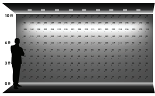
NINE LUMINAIRES 2'-0" away from wall 2'-0" between luminaires
