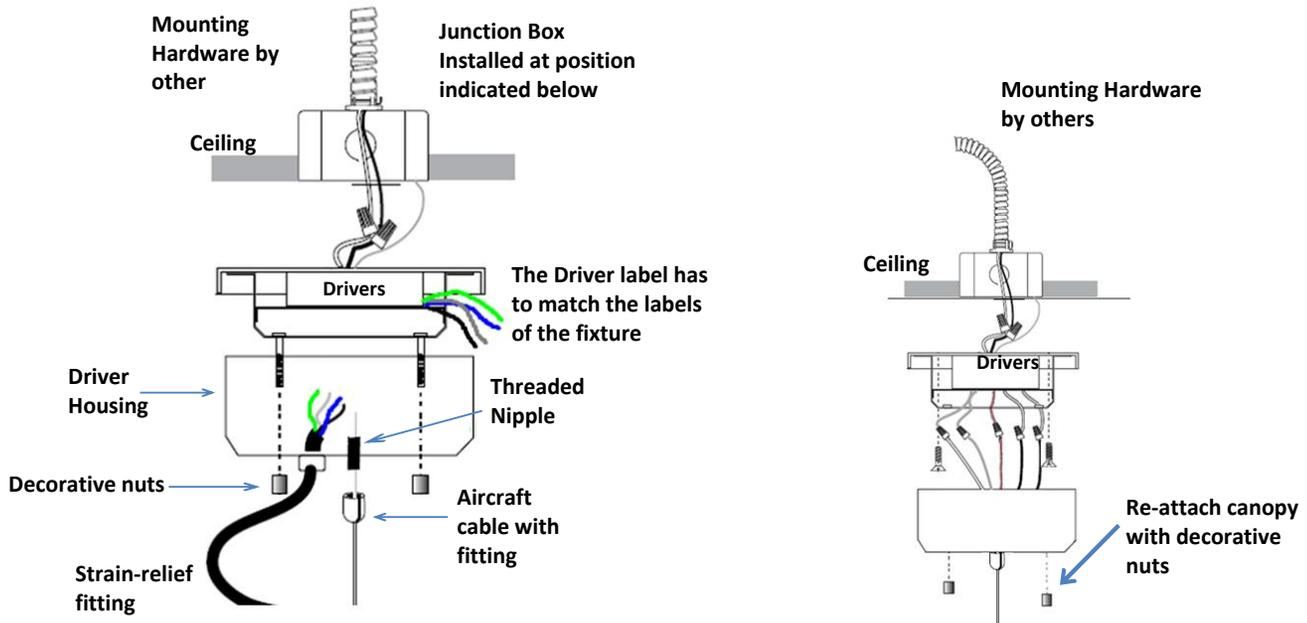
Before starting the installation, unscrew the two decorative nuts of the Driver Housing (factory provided). Then loosen the two nuts (Factory provided) holding the Driver Assembly with the Canopy.
