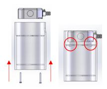
4. Attach the cylinder directly to the junction box using screws (supplied by others).
