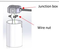
3. Make wiring connections from fixture to junction box.
