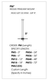
\*MAXIMUM ONE PIECE STEM LENGTH IS 72". LONGER LENGTHS ARE POSSIBLE USING MULTIPLE STEMS AND COUPLERS.
