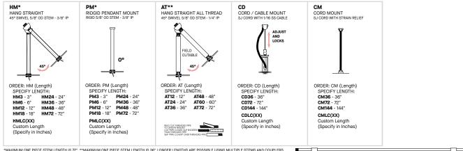
\*\*\* MAXIMUM ONE PIECE STEM LENGTH IS 72". \*\* MAXIMUM ONE PIECE STEM LENGTH IS 36". LONGER LENGTHS ARE POSSIBLE USING MULTIPLE STEMS AND COUPLERS. \*\* ORDER IN 12" INCREMENTS. ODD SIZES MAY BE FIELD CUT
