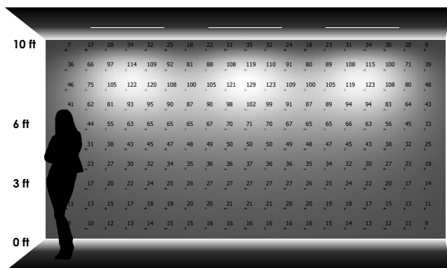
THREE LUMINAIRES 2'-0" away from wall 6'-0" on center
