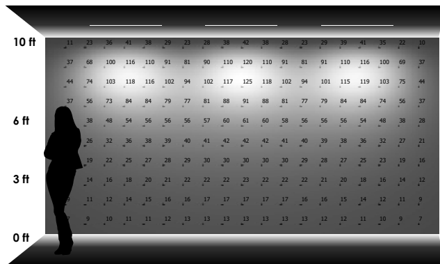
THREE LUMINAIRES 2'-0" away from wall 6'-0" on center
