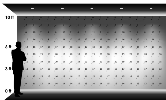
5 LUMINAIRES 3' - 0" away from wall 4' - 0" between luminaires
