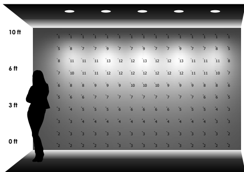
5 LUMINAIRES 3' away from wall 3' between luminaires
