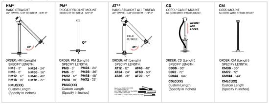
\*MAXIMUM ONE PIECE STEM LENGTH IS 72". \*\*MAXIMUM ONE PIECE STEM LENGTH IS 36". LONGER LENGTHS ARE POSSIBLE USING MULTIPLE STEMS AND COUPLERS. \*\*ORDER IN 12" INCREMENTS, ODD SIZES MAY BE FIELD CUT
