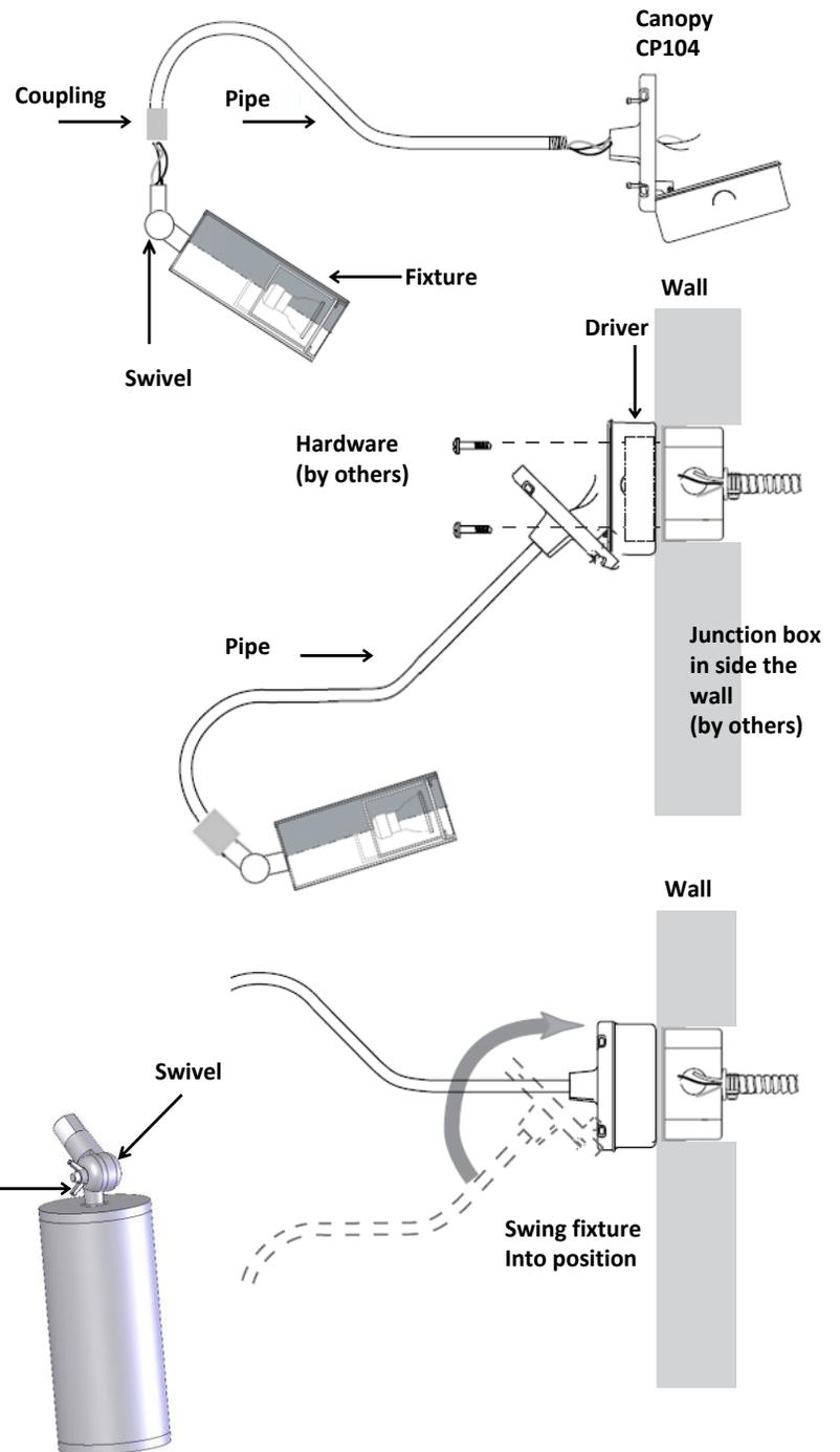
**Note:** Wrap threads with Teflon tape. Connections must be waterproof; Silicone – seal all pipe connections.
