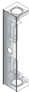
Detail: Key slots engage hardware at wall box. KO for Power Feed
