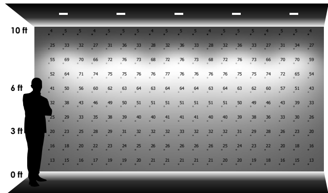
5 LUMINAIRE 3' - 0" away from wall 4' - 0" between luminaires
