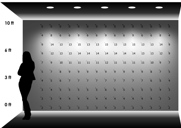
(5) ESO3RMF-930 013-D1-WW-MW A 3' AWAY FROM WALL B 3' BETWEEN LUMINAIRE
