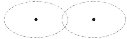
64° x 32° Beam Angles oriented for linear, overlapping light pattern
