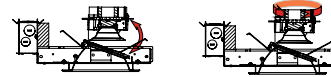
LED MODULE TILTS AND LOCKS TO 35° AND ROTATES AND LOCKS 360° WHILE MAINTAINING CENTER BEAM FOCUS
