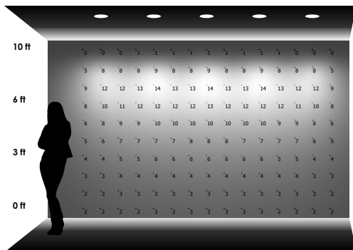
5 LUMINAIRES 3' away from wall 3' between luminaires
