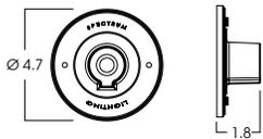
CUSTOM AND OTHER WALL ARMS AVAILABLE - CONTACT FACTORY. ARMS MAY BE FIELD CUT ON WALL SIDE - FIXTURE SIDE THREADED 3/4" NPT REQUIRES SEALANT FOR WET LOCATION.
