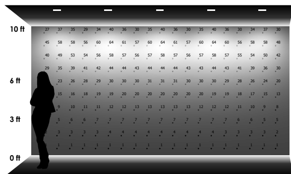
5 LUMINAIRES 4' - 0" away from wall 4' - 0" between luminaires 20° tilt towards wall
