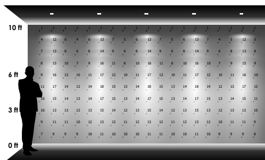
5 LUMINAIRES 3' - 0" away from wall 4' - 0" between luminaires
