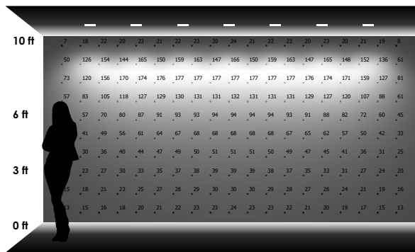
7 LUMINAIRES 2' - 6" away from wall 2' - 6" between luminaires
