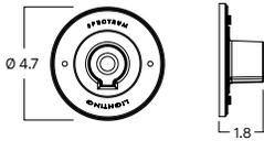
CUSTOM AND OTHER WALL ARMS AVAILABLE - CONTACT FACTORY. ARMS MAY BE FIELD CUT ON WALL SIDE - FIXTURE SIDE THREADED 3/4" NPT REQUIRES SEALANT FOR WET LOCATION.
