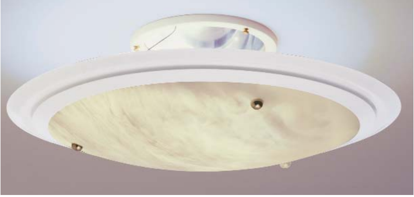
DSRB*-FA, DSRB*-WA, Suspended translucent bowl with formed metal ring. 16", 18", and 24" diameter. faux alabaster or white opal acrylic bowl. White, brass, brushed or polished aluminum ring finish. 8" or 9" apertures. (12" aperture 4" deep for low plenum). *specify diameter.
