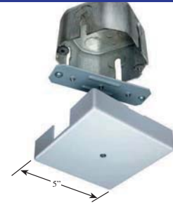
T-Bar Feed Kit Allows for feeding of track from an intersection point in a suspended ceiling application. For use with eco GES 11, 14, 34, 38, 39, 40 connectors. GES 17(-2,-3) 1 & 2 Circuit
